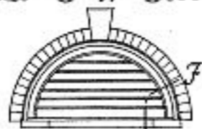
Louvred Opening in N.E. Pediment
